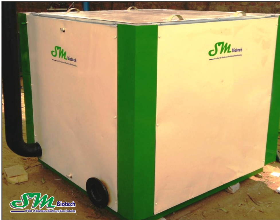
Straw Pasteurization Tank
