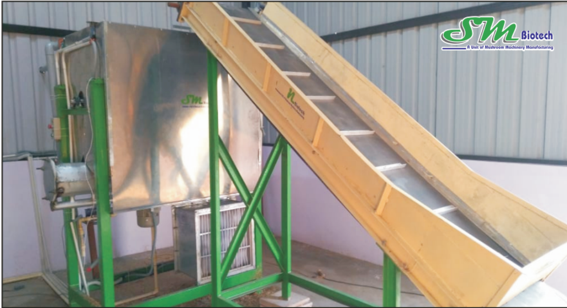
Straw Pasteurization Conditioning & Bag Filling
